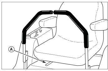
Figure 20. Seat Adjustment A. Seat Adjustment Lever
